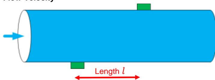
$$v_{meas} = c \cdot \frac{l}{2} \cdot \left( \frac{1}{tt_{down}} - \frac{1}{tt_{up}} \right)$$
